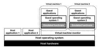
Figure 1. A standard structure for VMM, providing the abstraction of multiple VM-es.
